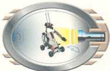
When a light is flashed L-8GO turns backwards and picks up speed.
