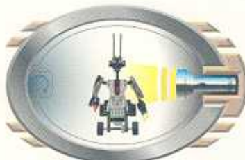
When L-8GO detects two flashes from a light source, the Robot changes direction.
